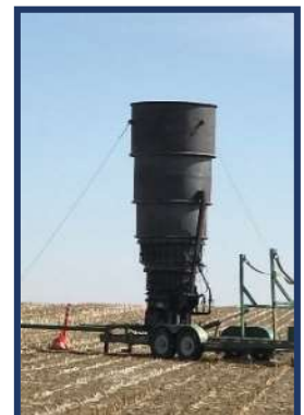
Emission Control Device (ECD)
