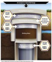
A drilling rig begins the underground construction process by installing steel pipe and cement (surface casing) to protect groundwater. Surface casing is set at least 50' below the aquifer, which is typically about 1,000' below the surface.
