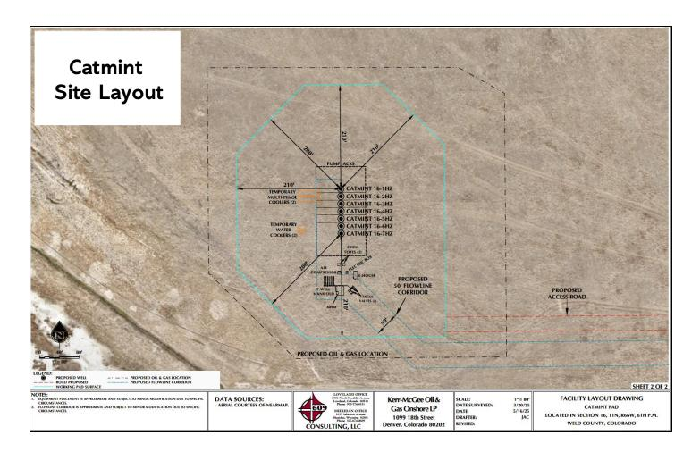
This proposed site layout shown above is currently being planned but is subject to change based on constraints, feedback, timing, etc. All 6 of the wells will be drilled from the surface location and run south.
