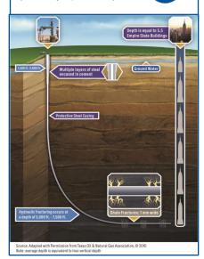
A production rig arrives and drills to a depth of 7,000 to 8,000 feet. The horizontal portion of the wellbore can extend more than two miles. Additional layers of protective steel casing and cement
