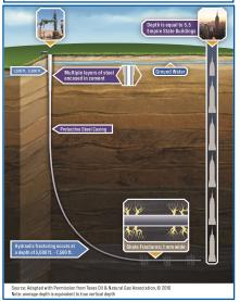
A production rig arrives and drills to a depth of 7,000 to 8,000 feet. The horizontal portion of the wellbore can extend more than two miles. Additional layers of protective steel casing and cement are installed.
