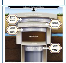
A drilling rig begins the underground construction process by installing steel pipe and cement (surface casing) to protect groundwater. Surface casing is set at least 50' below the aquifer, typically about 1,000' below the surface.
