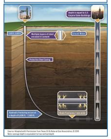
A production rig arrives and drills to a depth of 7,000 to 8,000 feet. The horizontal portion of the wellbore can extend more than two miles. Additional layers of protective steel casing and cement are installed. Well Completions (6-9 days per well)
