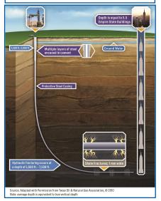
A production rig arrives and drills to a depth of 7,000 to 8,000 feet. The horizontal portion of the wellbore can extend more than two miles. Additional layers of protective steel casing and cement are installed.
